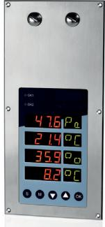
PMDS4 is a suitable positive and negative pressure monitoring of non-aggressive gases in cleaning rooms. Due to the construction of the device it can be directly installed into the partition. Up to four additional sensors for temperature and humidity can be connected to the device and displayed. The calibration and adjustment is made simply by using the front panel.
